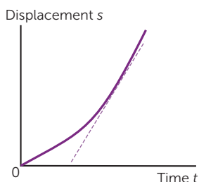
Fig. 2.22 Displacement versus time for an object released in a fluid
